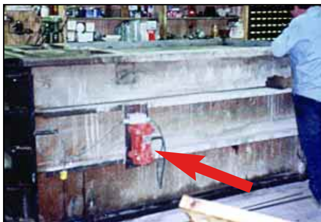
Model US-1600 permanently mounted on 5500 lb. mold.
