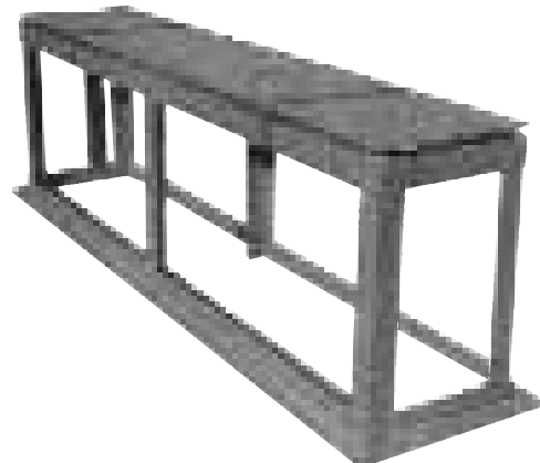
12' long vibrating table to handle multiple forms
