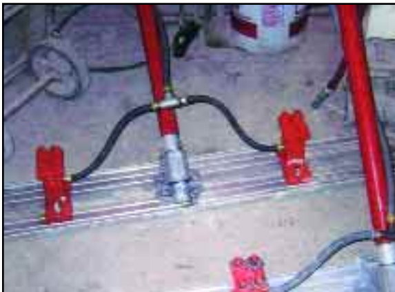
Screed with Model 50-1-1/4 pneumatic piston vibrator
